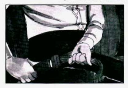
Buckle, position and release it the same way as the lap part of a lap-shoulder belt. If the belt isn't long enough, see "Safety Belt Extender" at the end of this section.
